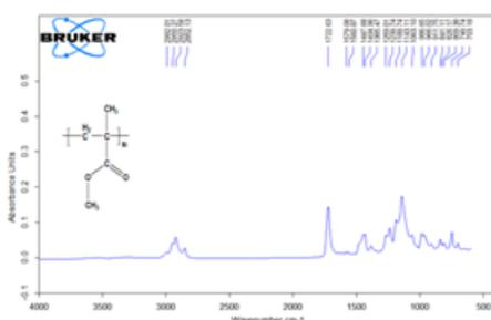
Figure (3): FTIR Spectrum that obtained for the Cold Cure PMMA Specimens.
