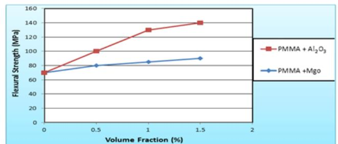
**Figure (8): Flexural Strength of PMMA Composite Materials as Function of ( $Al_2O_3$  or MgO) nanoparticles content in Composite.**
