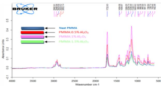
**Fig (5) FTIR spectrum of (PMMA: x% Al<sub>2</sub>O<sub>3</sub>) polymer composite as a function of nano-alumina content in composite**
