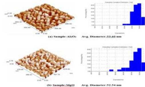
Figure (2): AFM Test of Nano (a)  $Al_2O_3$ (b) MgO
