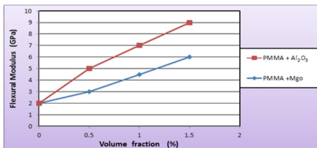
Figure (9): Flexural Modulus of PMMA Composite Materials as Function of (Al<sub>2</sub>O<sub>3</sub> or MgO) nanoparticles content in Composite.
