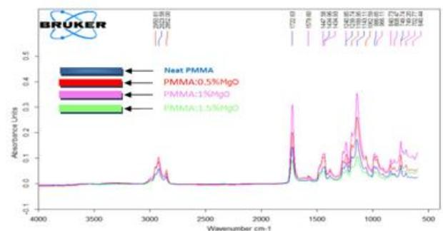
**Fig (7) FTIR spectrum of (PMMA: MgO) PMMA Nano composite as a function of nano-MgO content in composite**
