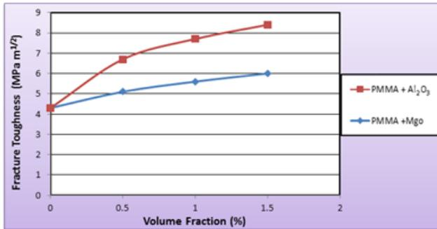
**Figure (11): Fracture Toughness of PMMA Composite Materials as Function Of (Al<sub>2</sub>O<sub>3</sub> or MgO) nanoparticles content in Composite.**
