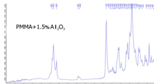
Figure 4: FTIR Spectrum that obtained for the polymer composite (PMMA: 1.5%  $\text{Al}_2\text{O}_3$ ) Specimens.
