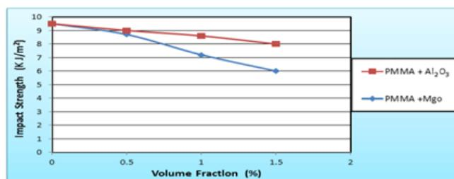
Figure (10): Impact Strength of PMMA Nano composite Materials as Function of (Al<sub>2</sub>O<sub>3</sub> or MgO) nanoparticles content in Composite.
