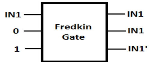
Fig.7. Single Fredkin Gate as 1:2 Decoder
