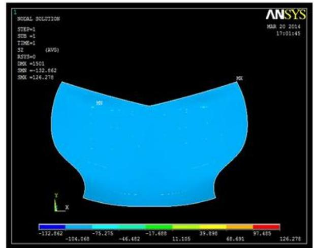
**Fig 15: Stress in z-direction**
