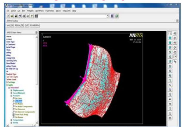
**Fig 11: Applying pressure on bonnet**
