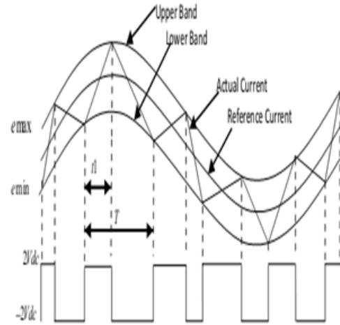
**Fig:4.2 Waveform of Hysteresis current controller**
