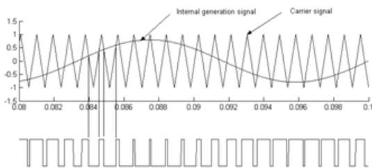
**Fig:4.1 Waveform of pwm current controller**
