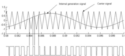
**Fig:4.1 Waveform of pwm current controller**
