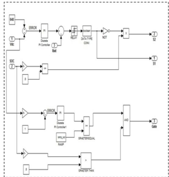
**Fig 5.9 Working Logic of Battery Operation**
