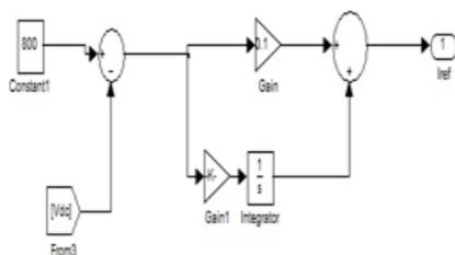
Fig.5.2 MATLAB Simulink model of PI control
