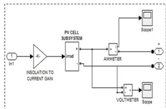
Fig 5.5 Transition Of Insolation Into Current Gain
