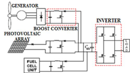
Fig 5.3 Model Of Proposed Hybrid Circuit
