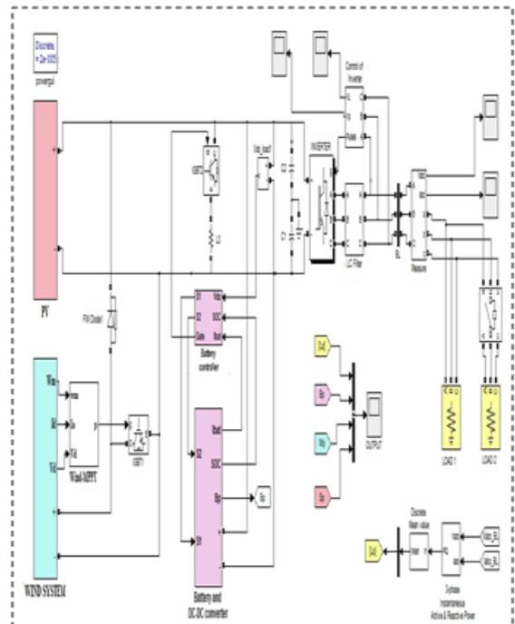
**Fig 5.10 Composite Simulation Model of Proposed Hybrid System**
