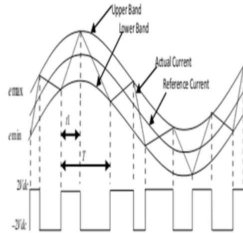
**Fig:4.2 Waveform of Hysteresis current controller**
