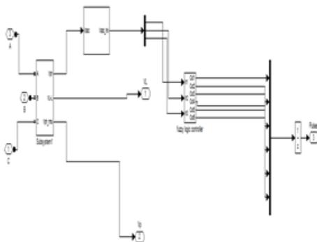
**Fig. 5.13 Fuzzy logic controller based pwm controller**
