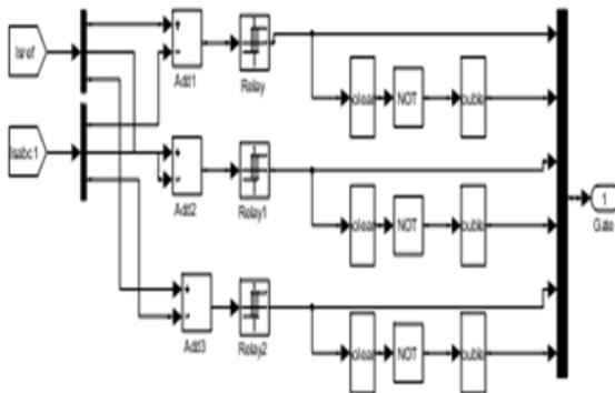
Fig. 5.1 Simulink Model of Hysteresis Current Control
