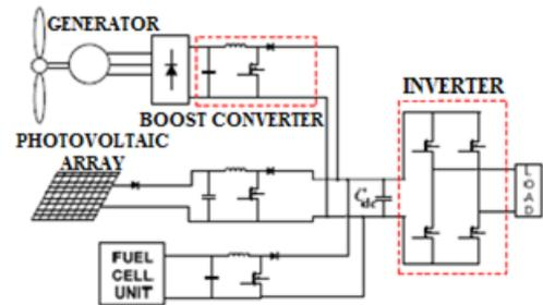
**Fig 5.3 Model Of Proposed Hybrid Circuit**
