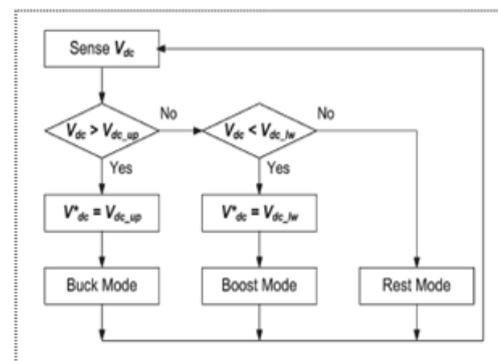
**Fig. 3.1. Battery-mode control block (modified hysteresis).**
