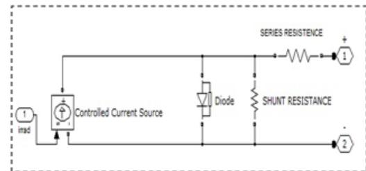
**Fig 5.4 Basic Structure Of PV-Cell**
