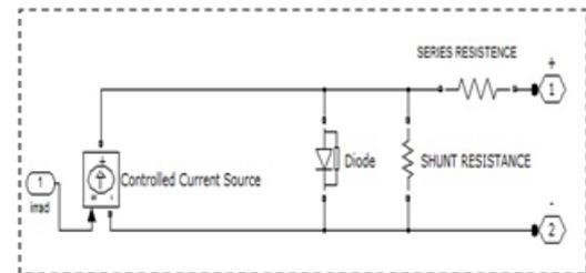
Fig 5.4 Basic Structure Of PV-Cell
