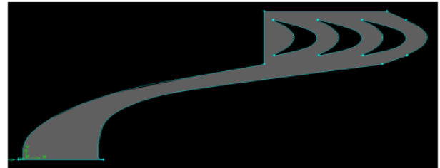
FIGURE Solid Model as a Partial Admission Case of Nozzle and Rotor Blades with 3mm axial gap.
