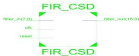
Fig 9: RTL Schematic of FIR filter
