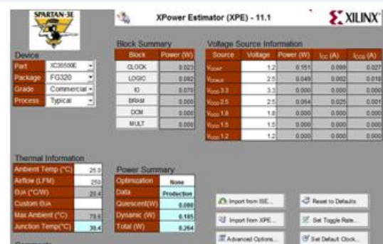
Fig 14: Power estimator of FIR filter with CSD algorithm
