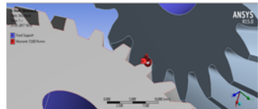
Fig 4.8 - : Contact stress on contact region
