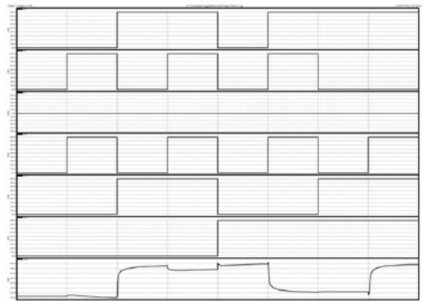
Fig. 9. Waveform of 1-bit ALU
