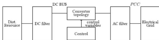
Fig. 5. Simplified layout for design.
