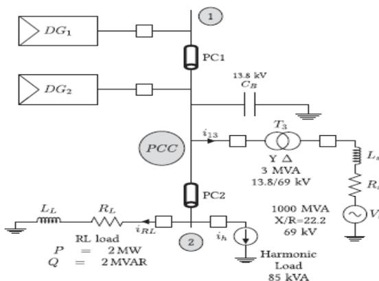
Fig. 6. Microgrid test system.
