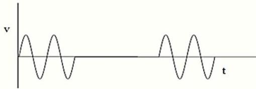
Fig.1 Voltage Signal with Long Interruption
