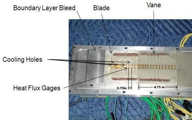
**Figure 5: Instrumented Flat Plate**
