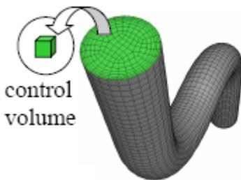
Fluid region of pipe flow discretized into finite set of control volumes (mesh).
