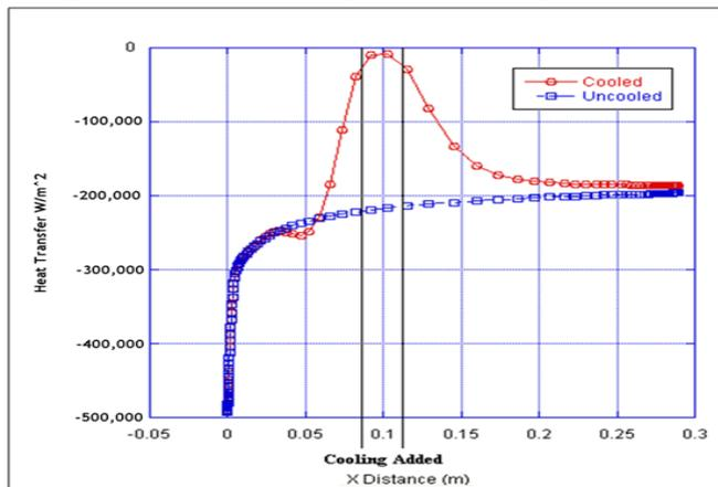
**Figure 17: Comparison of Single Block Cooled and Uncooled Heat Transfer**
