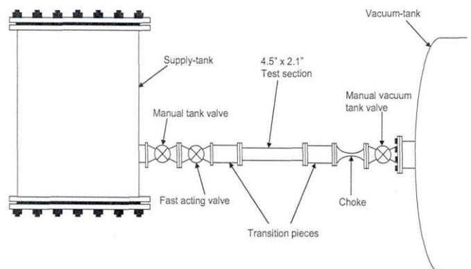
**Figure 3: Test Section Containing Flat Plate**
