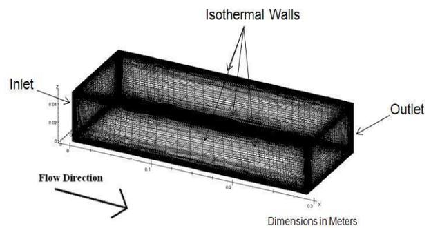
**Figure 6: Single Block Wall Boundary Conditions**
