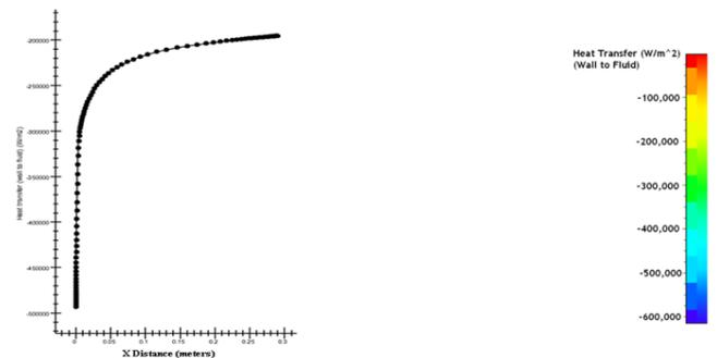
**Figure 13: Uncooled Single Block Heat Transfer Graph**
