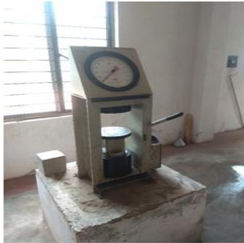
Compressive testing machine (Fig a)
