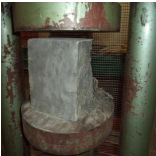
Figure.5.1.1: Crushed specimen after test
