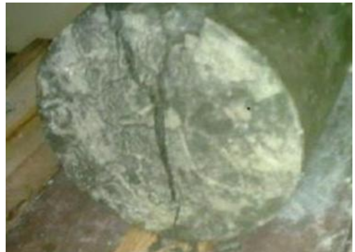
Figure 5.2: Specimen after being subjected to split tensile strength
