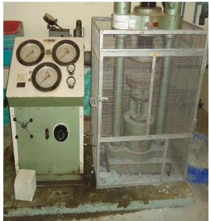
Figure.4.1: Test setup for compression test
