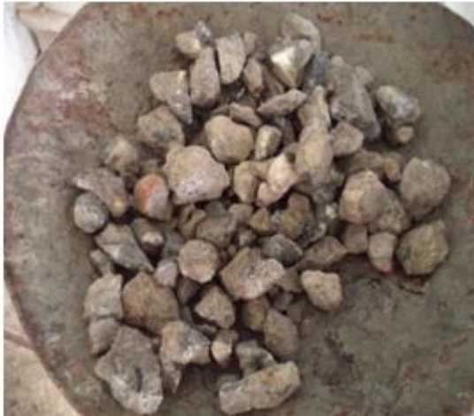
Fig.3.1: Crushing and washing of demolished concrete
