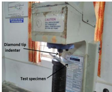
Fig. 4.7.5 (a): Rockwell Test machine with test specimen
