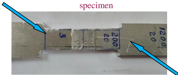
Fig. 4.7.5 (b) - Test specimen with indentation marks
