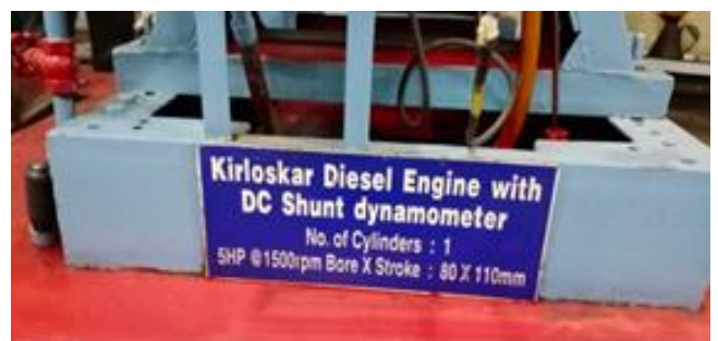
Figure 1.2: Details of Single Cylinder Kirloskar Engine
