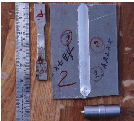
Fig 1 Dissimilar metals AA2024 and AA7075 Al welded alloy sheets with tensile sample and FSW tool.
