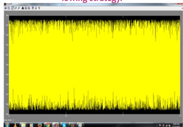
Figure 11: DC-link voltage ( v_{dc} ) of HPS under grid following strategy.
