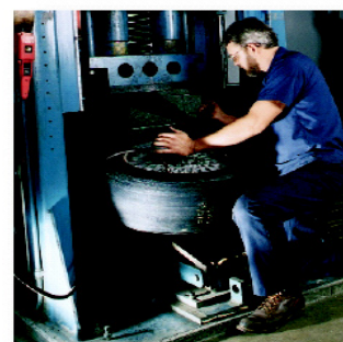
Wheel being prepared for Impact Test. Our procedures meet (or exceed) SAE, SFI, ISO, and JASCO requirements.
