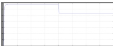
Fig.11. simulation result for speed of PMSG under variation speed
