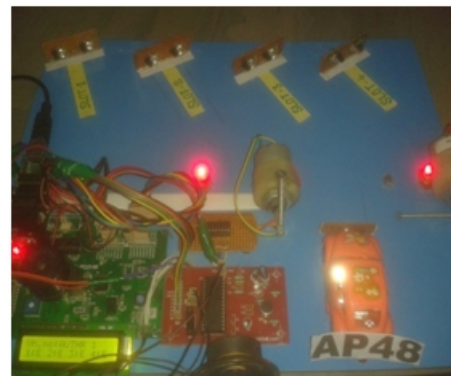
Fig.7.3: The authorized vehicle can be allotted for the slot-1 and opens the entrance gate.
