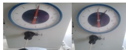
Fig.9: Minimum Torque output- 42kgm, Fig.10: Maximum Torque output- 148kgm
