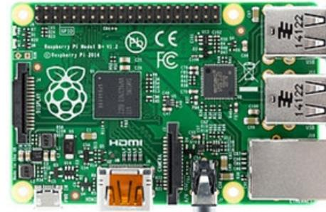
**Figur3: Raspberry Pi Board**
