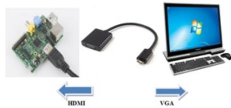
Figure9: HDMI to VGA cable connection
