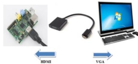
Figure9: HDMI to VGA cable connection
