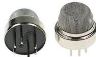
Fig7:Gas Sensor (type-MQ2)
