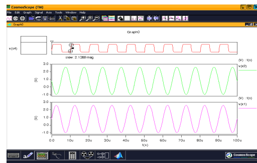
Fig.5: Simulation results for Conventional two-stage miller op-amp
