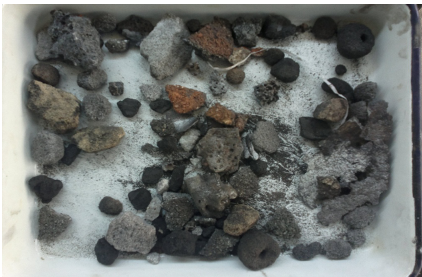
Fig: 2 Deleterious Materials in WFS
