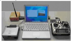
The control loop, shown in Figure, starts with collecting all the sensor and video data, and they are streamed back to the ground station from on-board computer. After these data are processed, control commands will be sent back to the airplane by a custom interface and the trainer function on a Futaba RC controller, which allows switching between computer and human control instantaneously
