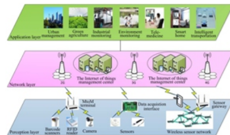
Figure1: Architecture of IOT.
