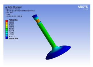
STRUCTURAL ANALYSIS POPPET VALVE WITH TECHNETIUM MATERIAL
