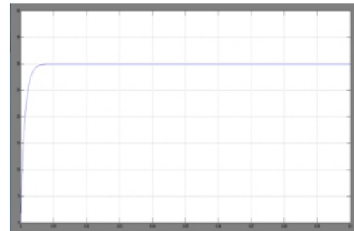
Fig: simulation waveform of output voltage for closed loop system with flying capacitor
