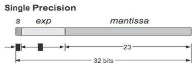
Figure1. Single Precision Floating Point Format.
