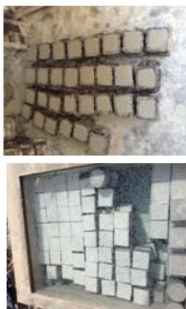
Fig 4. Casting & Curing of Specimens
