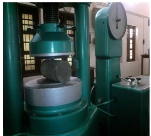
Fig: 8 Test for Splitting Tensile Strength
