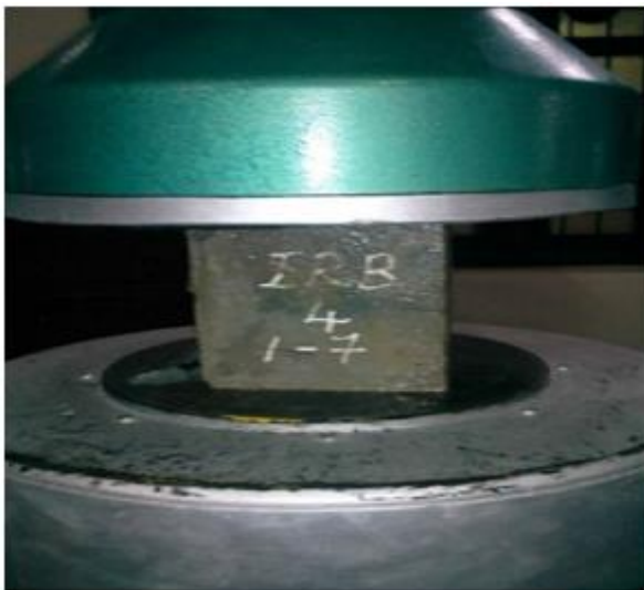
Fig: 6 Test for Compressive Strength
