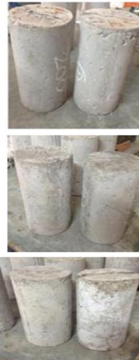
Fig.16. Colour change of M60 Grade Concrete of Basalt and Normal when exposed to 200°C, 600°C & at 800°C temperatures.
