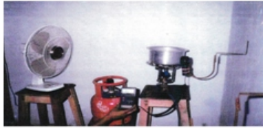
Fig: Test set up for Resistance to Draught
