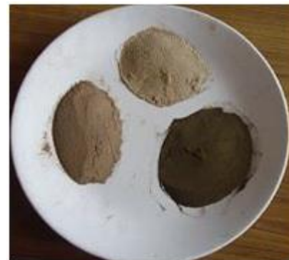
Figure 3.1.1: Samples of Groundnut Shells and Powder
