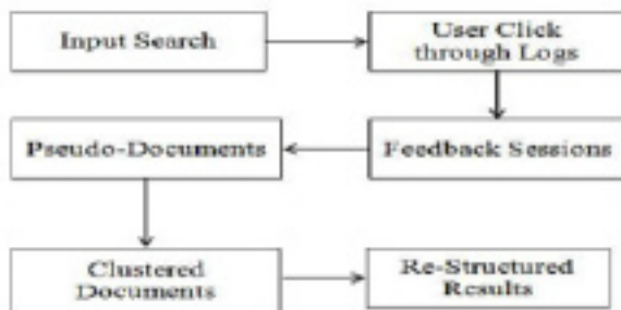
Fig:-overall data flow of the proposed system
