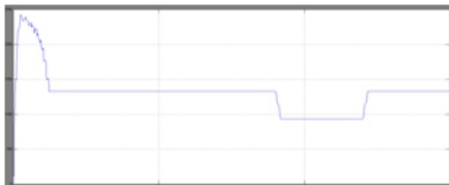
Fig.14. simulation result for RMS value of source voltage during sag
