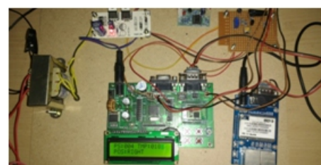
Figure 3 PCB development of Health Monitoring System
