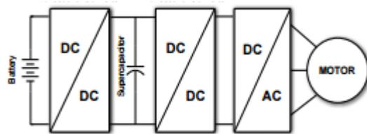
Fig. 4. Cascaded converter configuration
