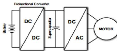
Fig. 3. Battery/ supercapacitor active configuration
