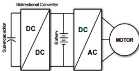
Fig. 2. Supercapacitor/ battery active configuration
