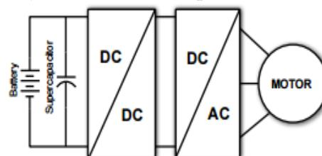
Fig. 1. Passive parallel configuration
