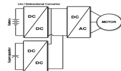
Fig. 5. Multiple parallel connected converter configuration
