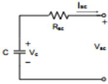
Fig. 9. The super capacitor model
