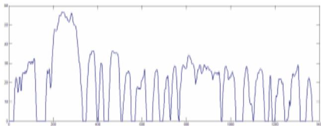
Fig. 7. Urban Dynamometer Driving Schedule (UDDS)
