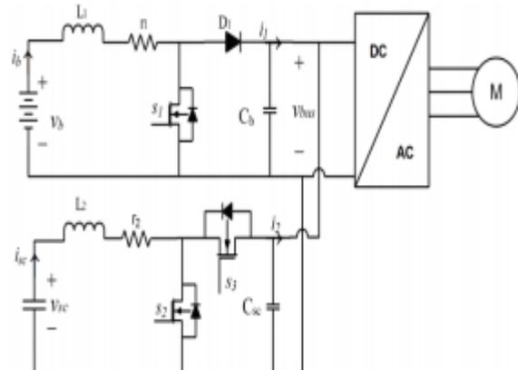
Fig. 6. Circuit level diagram of multiple parallel connected converter configuration
