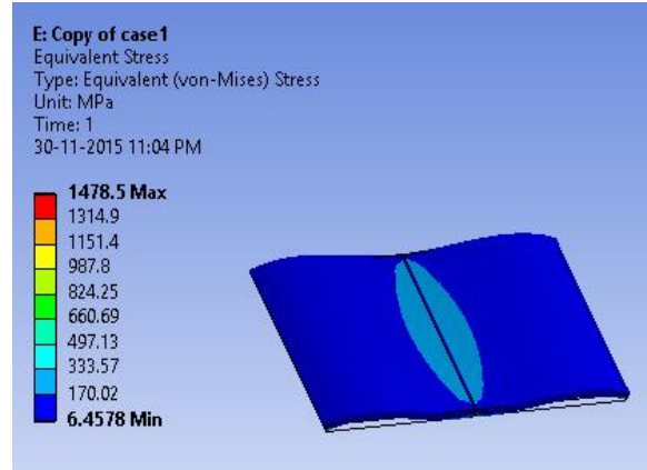
Fig3.9 von-mises stress of weld plate is 1478.5 MPa in 1st sec, without stamping condition in case-1.
