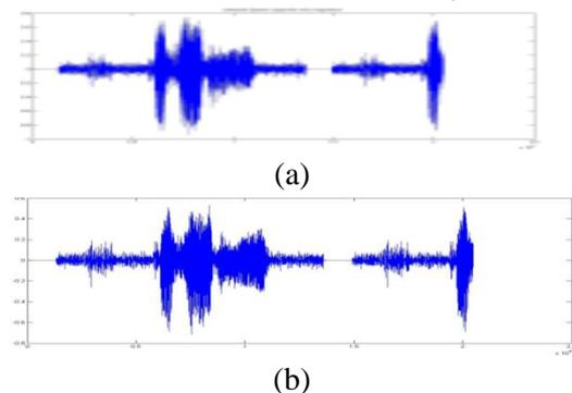
Fig10. (a) Original voice signal (b) De-noised signal for training
