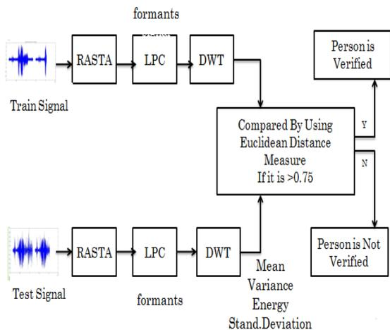
Fig9. Block diagram of proposed text dependent speaker identification system
