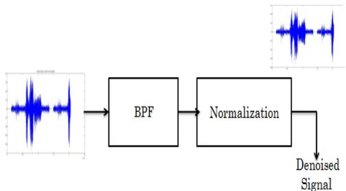
Fig.8 Block diagram of RASTA process
