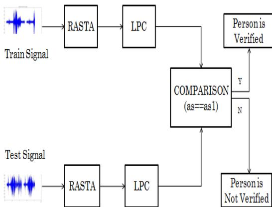
Fig6. Block diagram of LPC based recognition system
