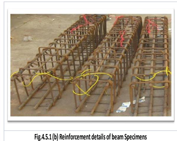
**Fig.4.5.1 (b) Reinforcement details of beam specimens**
