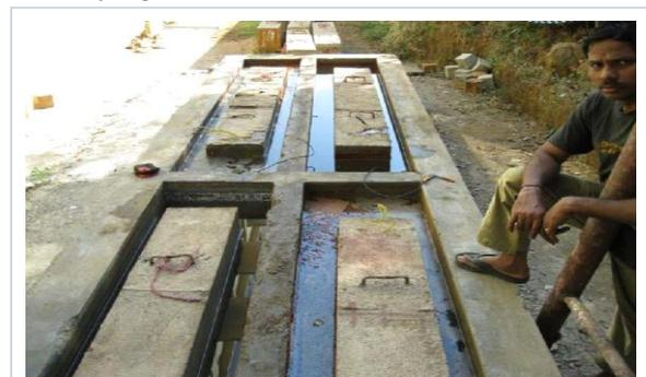
Fig.4.7.1 Photo of beam specimens under accelerated corrosion
