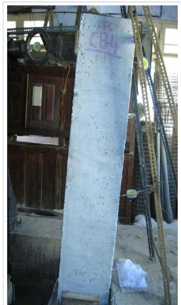
Fig.6.2 Deflection of beam after Flexure failure
