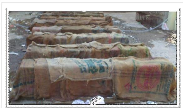
Fig.4.6.2 Curing of Beam Specimen
