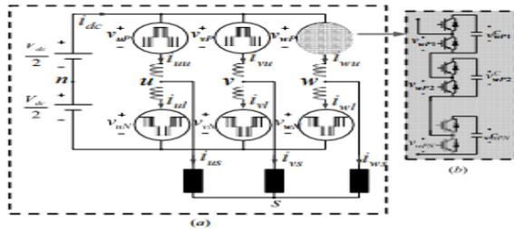
Fig. 1. Circuit configuration of the MMC
