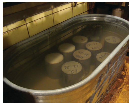
Fig (2) Curing of concrete cylinder
