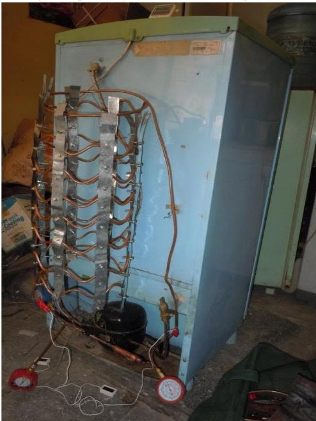
Fig 6 Proposed System with Pitch Angle 90° & Rectangular Shaped Fin.
