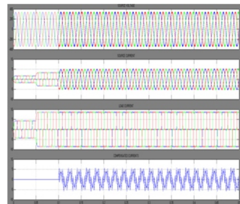
Fig.9. simulation results for (a) source voltage (b) source current (c) load current (d) compensated currents
