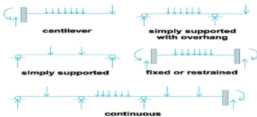
**Fig 1: showing the different types of beams.**
