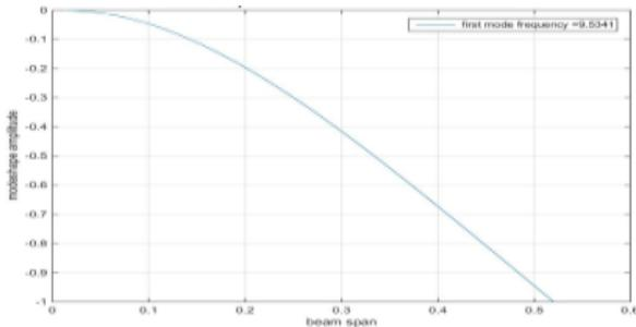
**Fig.6.1(a) :mode shape of the first mode**
