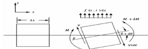
**Fig 4 Free body diagram of a section of a beam under transverse vibration**
