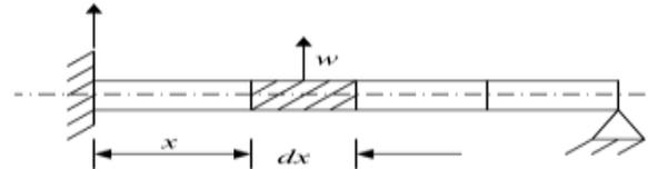
**Fig 3 A beam under transverse vibration**
