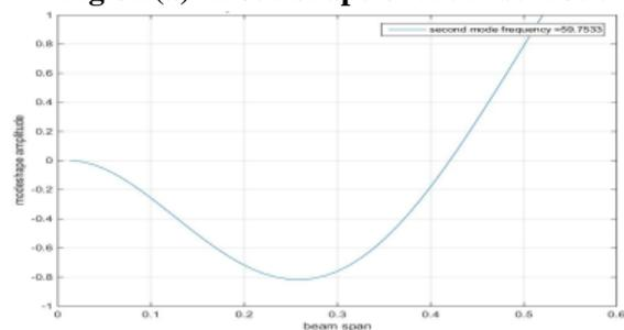
**Fig 6.1(b) : mode shape of the second mode**
