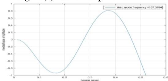
**Fig.6.1(c): mode shape of the third mode**
