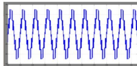
**Fig.9.Simulation results for output voltage of inverter with 2/3 Vdc.**
