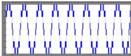
**Fig.12. Simulation results for output voltage of eleven level inverter.**
