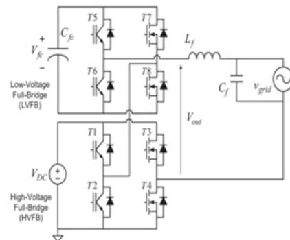
**Fig. 1. CFB with a flying capacitor**
