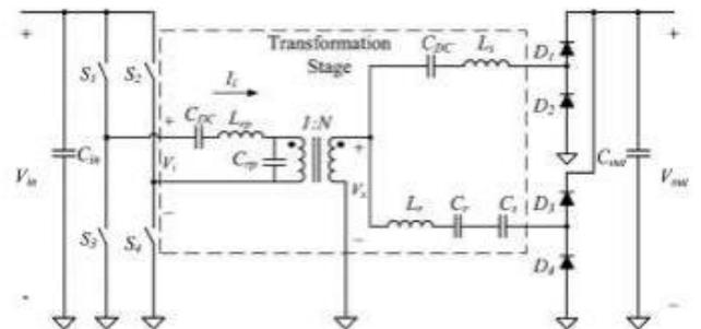
Fig. 2. Topology of the proposed RCN dc/dc converter.
