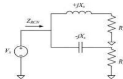
Fig.3. Fundamental frequency model of the RCN and the rectifiers
