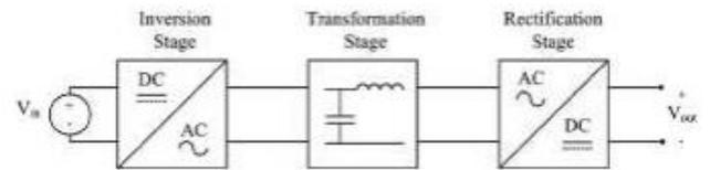
Fig. 1. Architecture of the proposed dc/dc converter.
