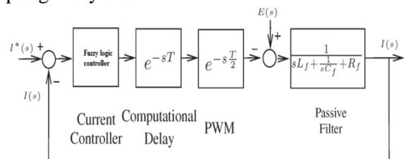
**Fig. 2. Closed-loop model of the current control.**
