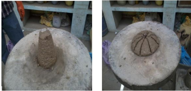
Fig 5.2- Flow of the Geopolymer mortar
