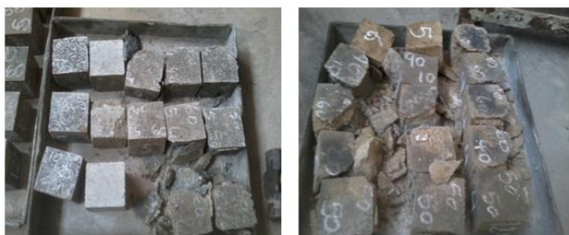
Fig 4.3 Cracking pattern of Geopolymer samples
