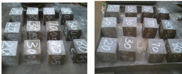
Fig 4.1 Samples of Geopolymer Mortar cubes
