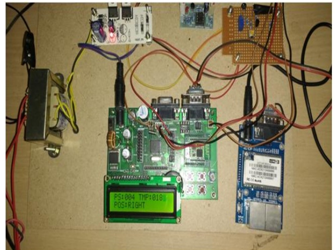
Figure 6.1 PCB development of Health Monitoring System
