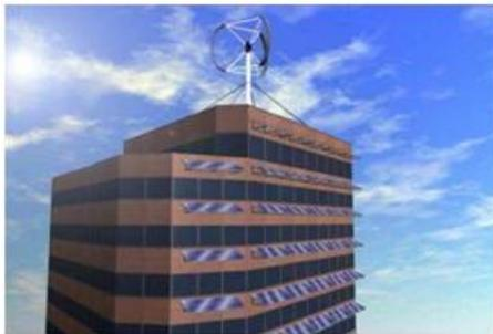
**Fig: 4.2** Wind and PV-based power generation for the vertically integrated microgrid.
